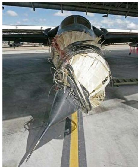
*Photo: The nose of the F-111 after the strike in April, 2009. Credit: RAAF*
