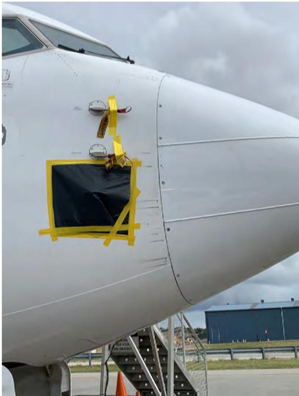
**Photo:** Aircraft at Perth Airport showing anti-wildlife storage protection - supplied
