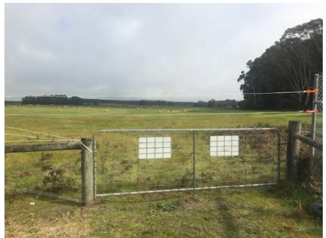
Photo: Mt Gambier airport's fence, showing the sprung gate hooks to allow easy access through the gate – supplied
