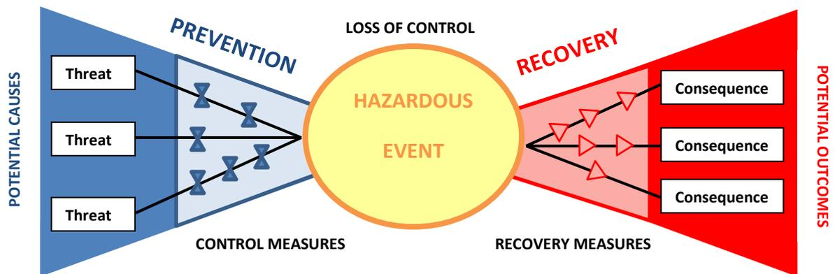
Figure 1.3: The basic structure of the bow-tie method
