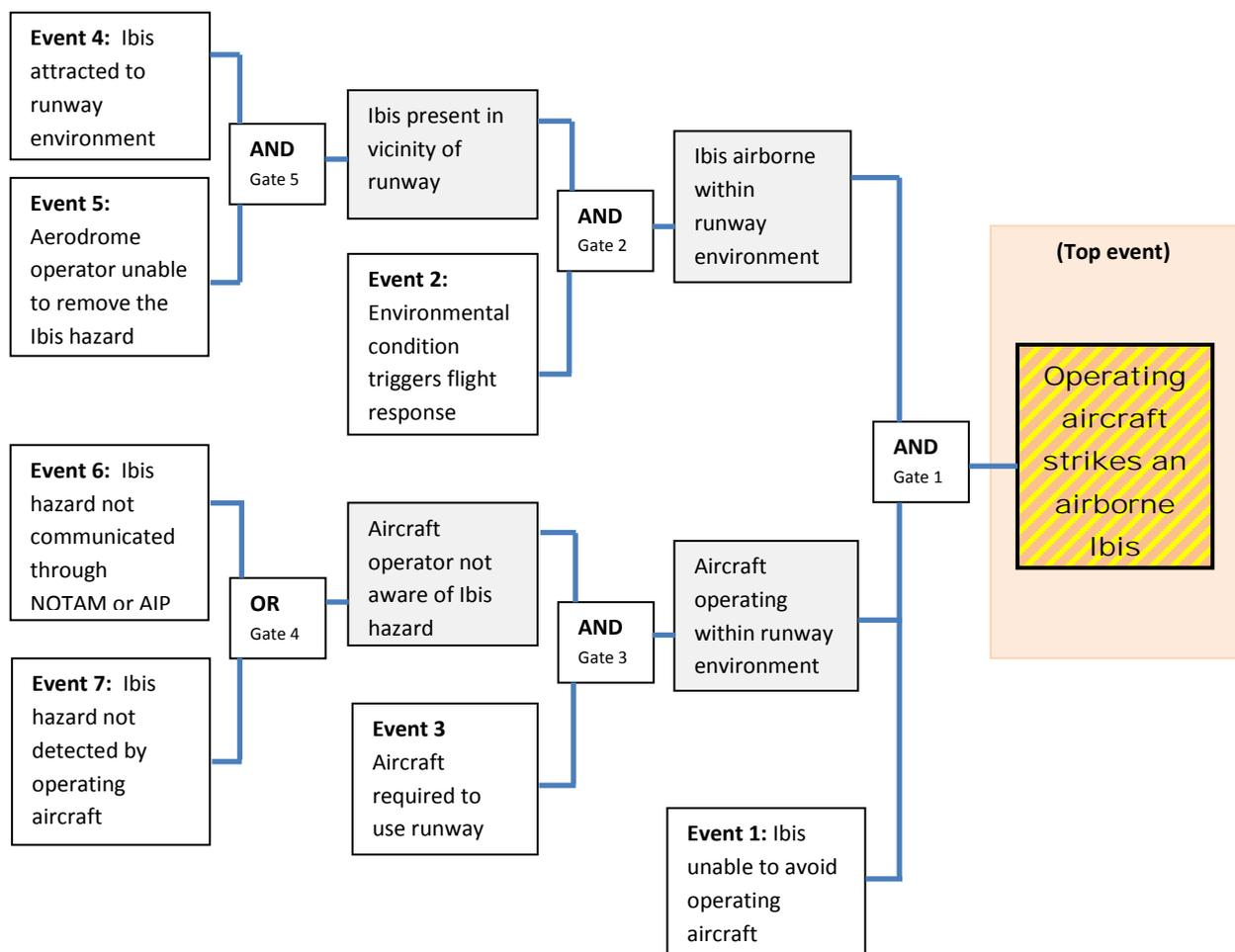
**Figure 1.5: Simple example of a Fault Tree Analysis method (for illustrative purposes only)**
