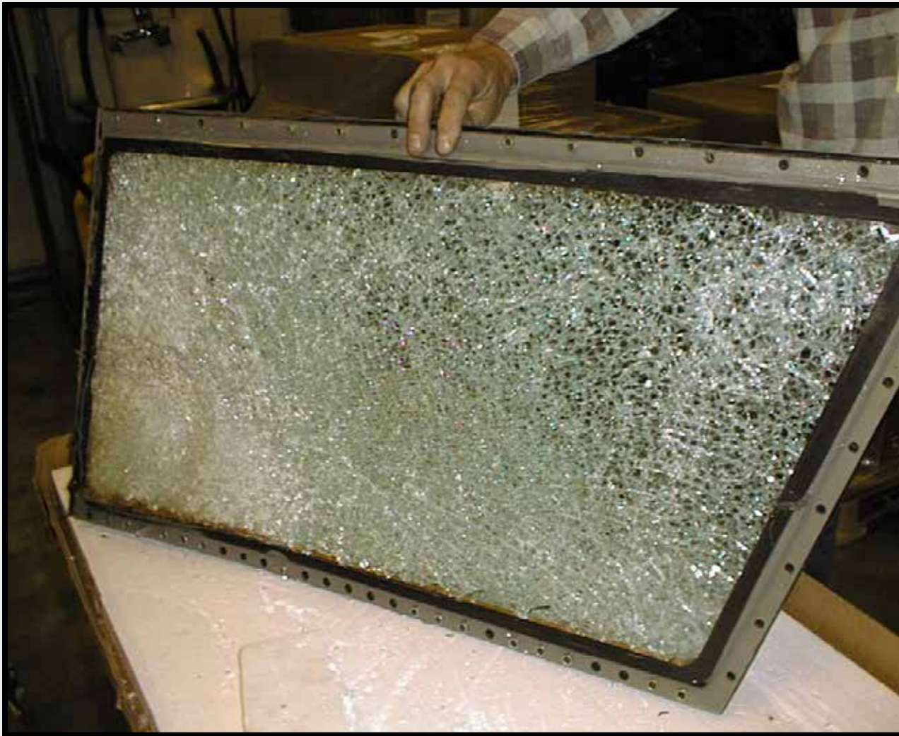
B-737 windshield destroyed by goose impact over New York – window spalled on impact showering cockpit with glass
